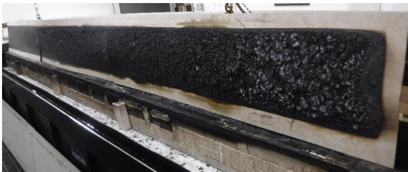
Photo No. 4 Exposed Surface of the Test Specimen (Post-test)
