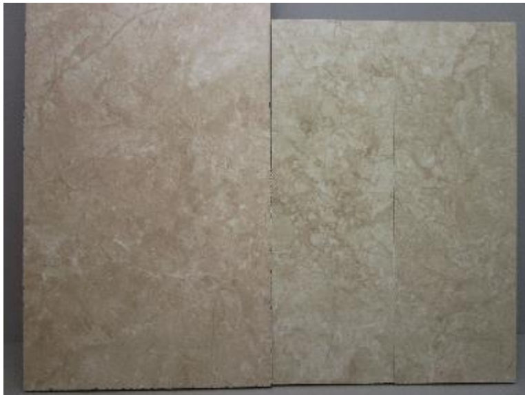
Photo No. 2 Section 4.1.1 - 2,005 Hours of Accelerated Weathering Control (Left); Aged Specimens (Right)
