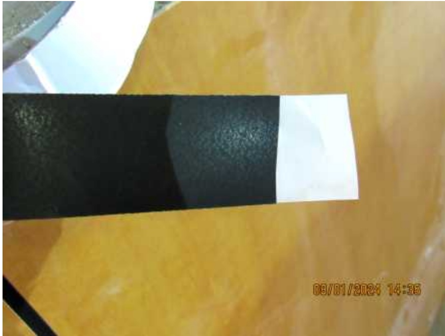
Photo No. 5 Intumescent Tape used Behind Panel Edges
