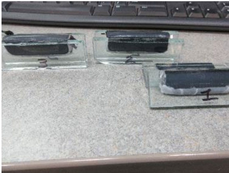
Photo No. 4 Test Result of Specimen 1 Complete Separation from Substrate.
