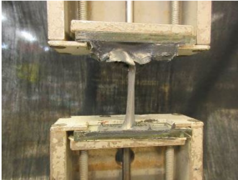
Photo No. 15 Specimen Undergoing Tensile Test
