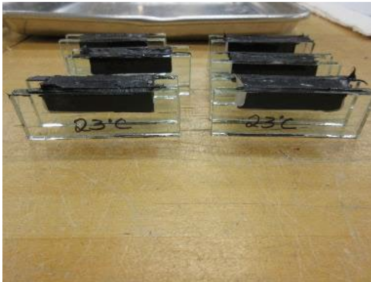
Photo No. 13 Lab Conditioned Tensile Test Specimen
