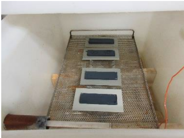
Photo No. 6 Hardness Test 7 Day Humidity Exposure
