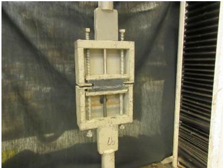
Photo No. 14 Tensile Test Setup
